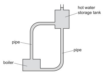
By which process does the heated water move up from the boiler to the hot water storage tank?
